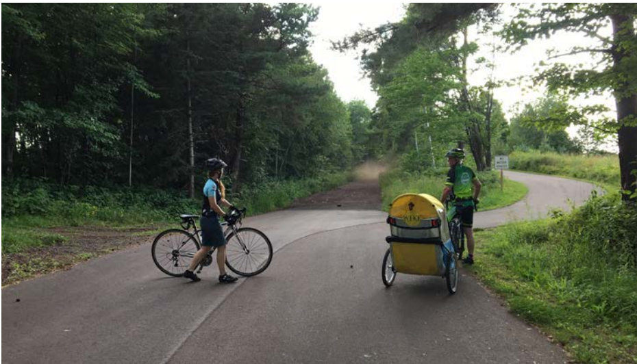
Non-motorized and motorized trails merge briefly in the Ironwood to Bessemer segment of the Iron Belle Trail. Note trails are paved side-by-side and double width to reduce user conflict.
