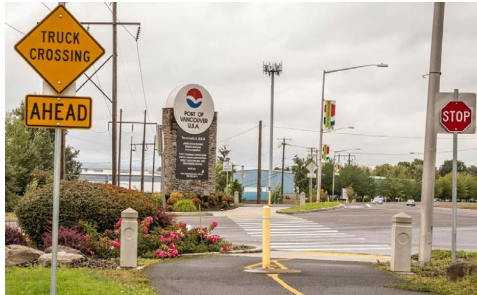
An example of a safe trail crossing with sidewalk enhancements such as signage, bollards, material change at crossing, and a designated crosswalk. Port of Vancouver Trail, Vancouver, Washington.
